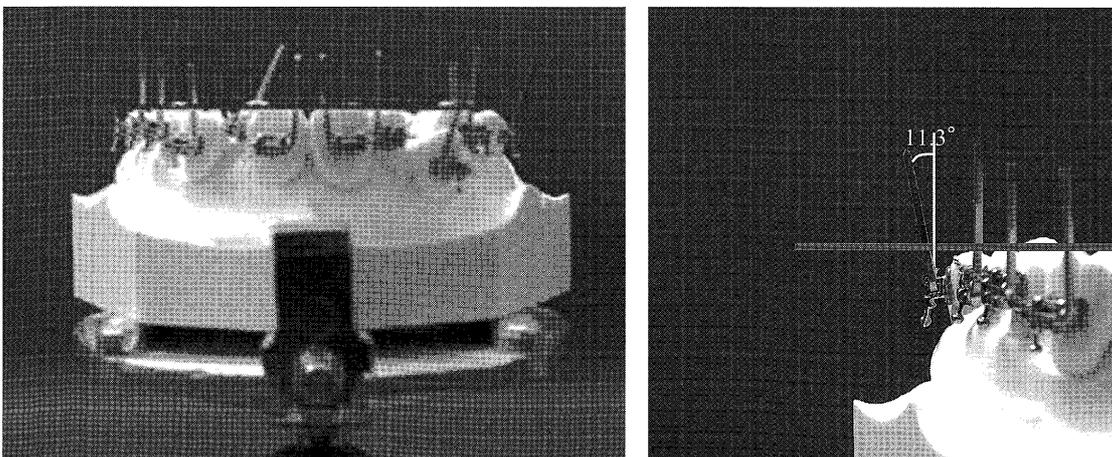
**Figure 4.** Predicted torsional angles. Small pieces of full size wires (0.0215×0.028inch) bent 90° were ligated. The predicted torsional angles was considered the perpendicular to the occlusal plane and the ligated wire.
