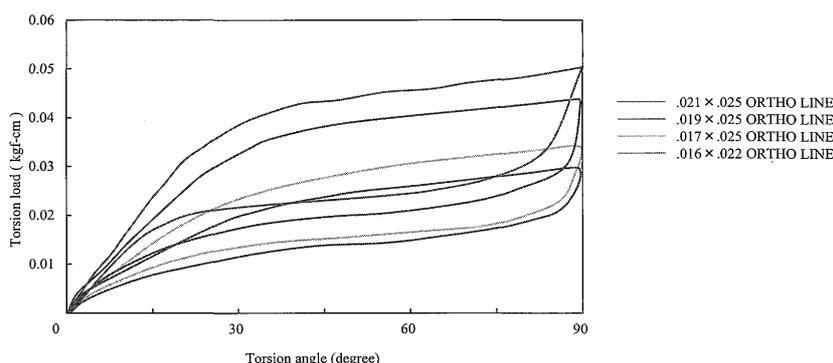
Figure 8. Representative torque-twist curves for ORTHO LINE with 4 different rectangular cross-sections.
