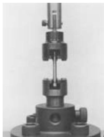
Fig. 2-3 Jig for the tensile test.
