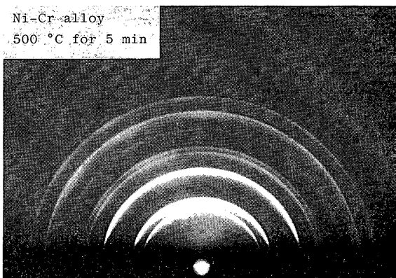
Fig. 9 Reflection electron diffraction pattern obtained from the specimen oxidized at 500°C.
