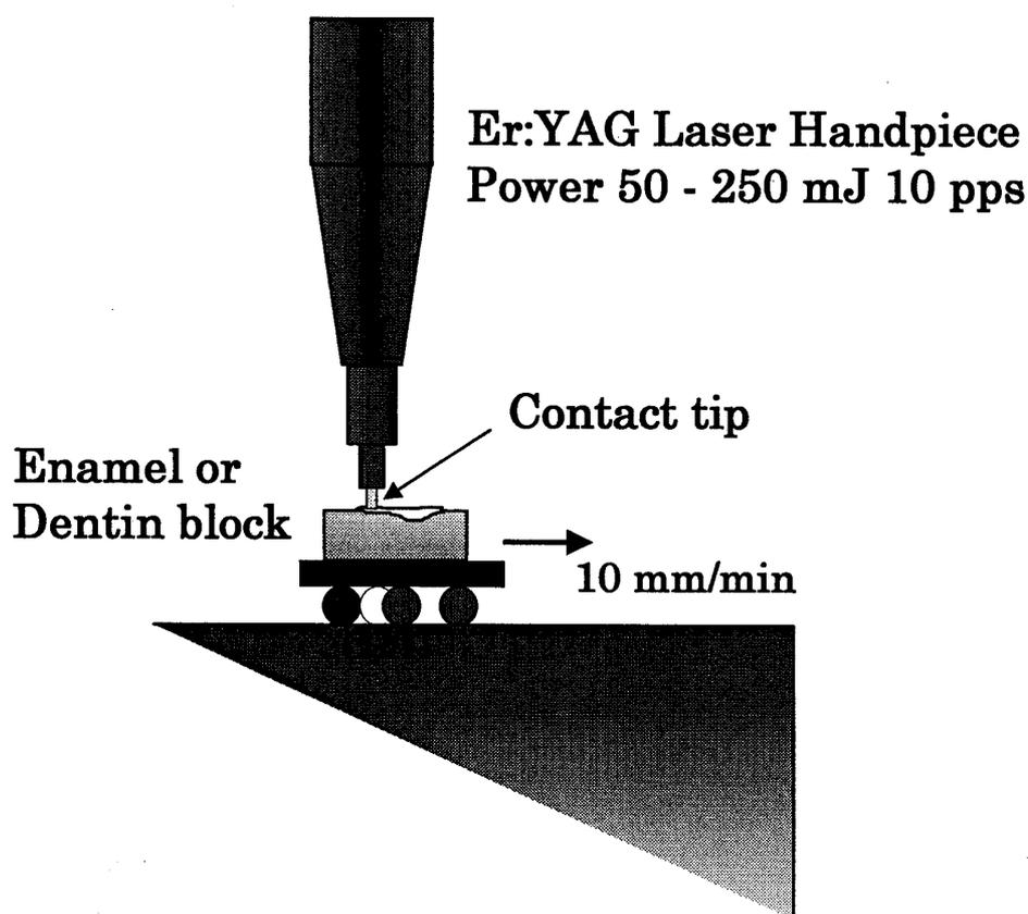
Fig. 2 Test method for cutting efficiency evaluation
